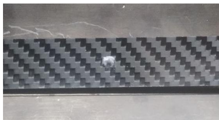
Fig. 3. A working part of a multi-layer woven T300 CFRP twill type sample damaged by a type IV impactor with an energy of 10 J.
