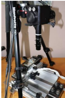
Fig. 1. Shearographic measuring system and test specimen of aluminum alloy.
