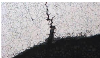
Fig. 1. Formation of pitting corrosion of steel links of the gas pipeline
