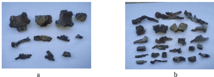
Fig. 2. Fragmentation of cylindrical Steel 45 specimens after explosive tests for hydrogen-free (a) and hydrogen-charged (b) specimen.
